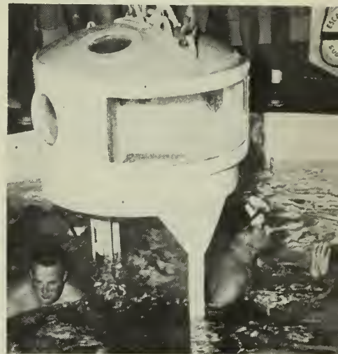
DIVING BELL is put to use in 100-foot tower for deep-water training.
